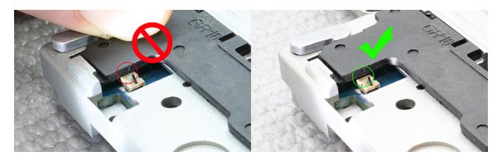
If the plate catches on the microswitch housing, use a gear shim to space the board away from the gearbox shell to give the plate proper clearance over the housing while still engaging the switch. The shim can be placed over the screw hole on the gearbox and then place the switchboard on top of it so that the screw which secures it passes through the center of the shim.
