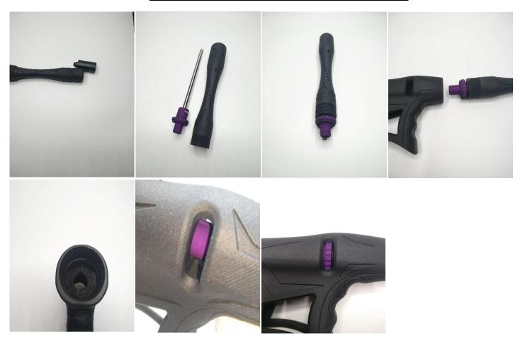
The tracer is located at the front of the outer barrel. To install it: screw it in an anti-clockwise direction and in a clockwise direction for its disassembly. (We recommend not to screw it too hard so that it remains easy to remove). Before screwing the outer barrel to the body of the ATOM make sure that the centering groove of the Hop-Up block is aligned with that of the body of the ATOM.
