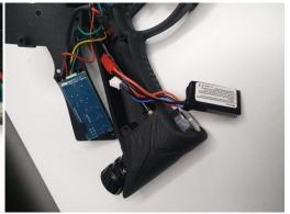
Cut the excess FCU thermal sheath if it bothers you. Connect the connectors to the FCU. Remove the preinstalled screw inside the ATOM pad, slide the POLARSTAR FCU into the slot, make sure everything is centered on the other side of the ATOM pad, then replace the screw in position. Install your battery and connect the connectors. Close the ATOM plate (be careful not to pinch the cables). Finally, replace the 4 screws of the ATOM plate.
