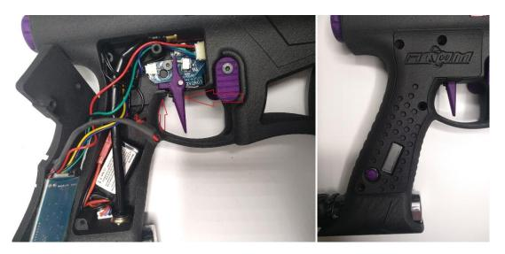
The trigger has two settings as shown in the picture, forward setting and backward setting. The settings are accessible from the outside of the ATOM, no disassembly needed. For maintenance, if you want to remove the trigger, you just have to pull on it, be careful, don't lose the small spring.
