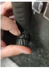
Regulator setting for power. Screwed the power decreases, unscrew the power increases.
